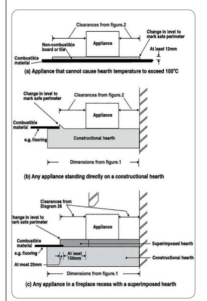
fig.3. Ways of Providing Hearths
