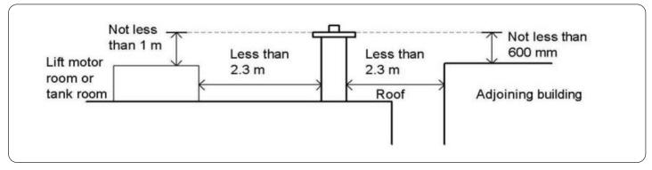
The Outlet of a chimney or flue in relation to an adjacent building should be as seen above
