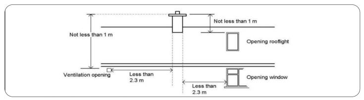
The outlet of a chimney or flue pipe should also be not less than 1m above the top of any opening skylight, opening window or wall ventilator within 2.3m
