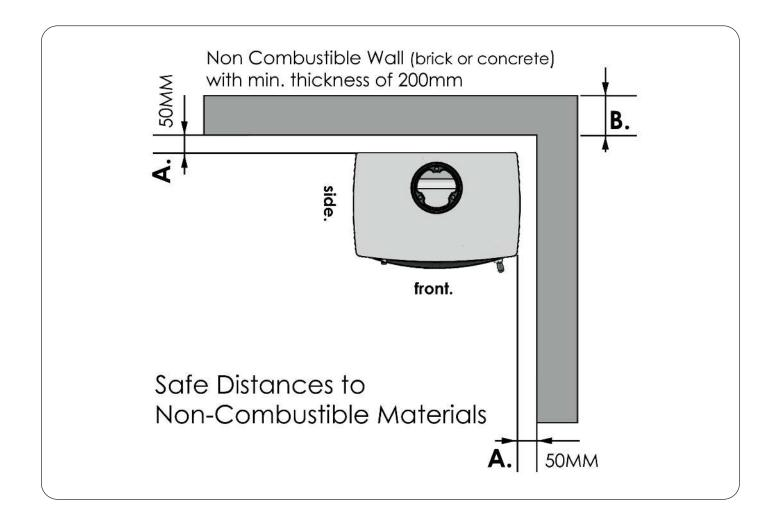
All stoves will require adequate distance between them & any non-combustible material to allow for both Installation & servicing, as well room for convection in order for the stove to operate correctly.
