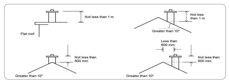
Outlet of a chimney or a flue to be not less that 1m above the highest point of contact of chimney and roof. Where the roof has a pitch of more than 10° on both sides and the outlet is at the ridge or within 600mm of it, the height of the chimney or flue pipe may be reduced to 600mm.
